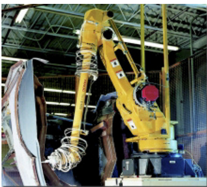
Precision robotic waterjet cutting is used to ensure part to part trimming accuracy.
